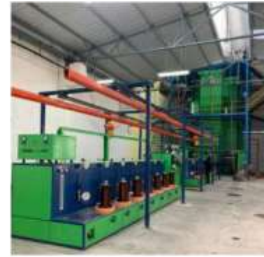
1. Vertical wire enamelling Machine 2. Make : Imported 3. Total Lines : 28 4. Wire range : 1.2 ~ 3.0 mm 5. Enamelling Application Method : Dye System ( 8 - 12 pass)
